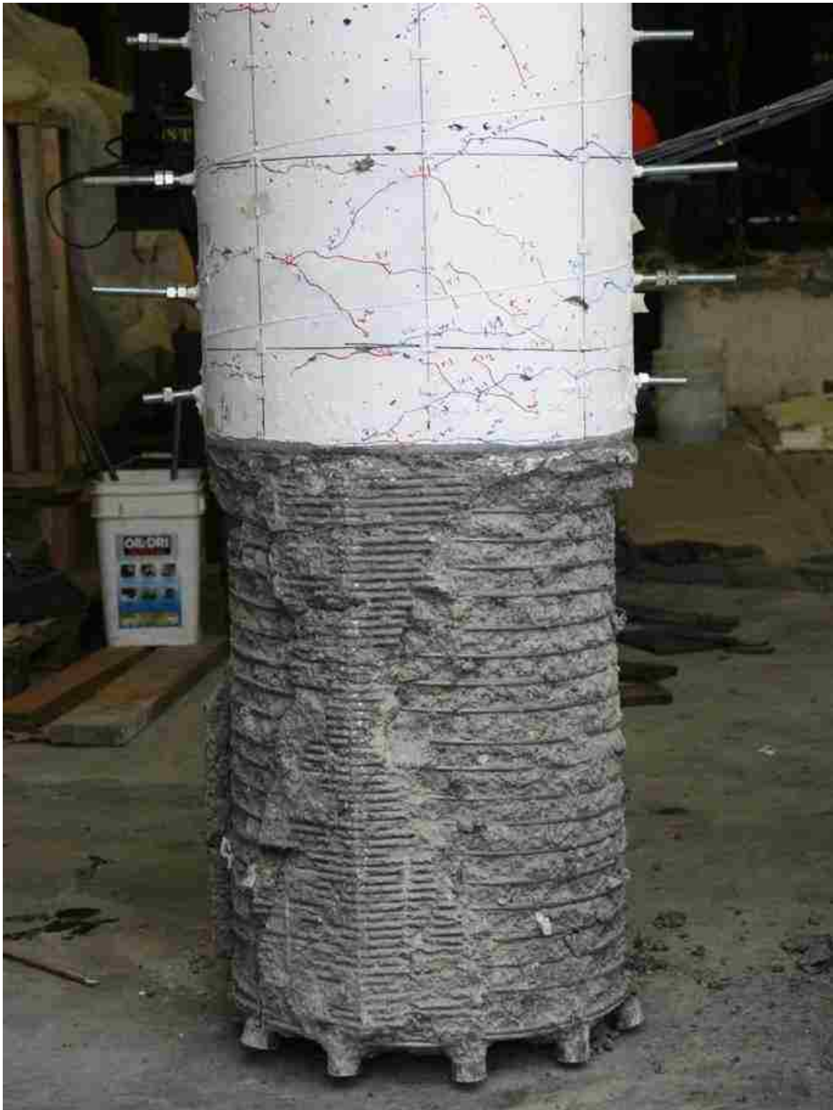
Figure C-0-13. DS-2 – Column damage after cyclic testing
