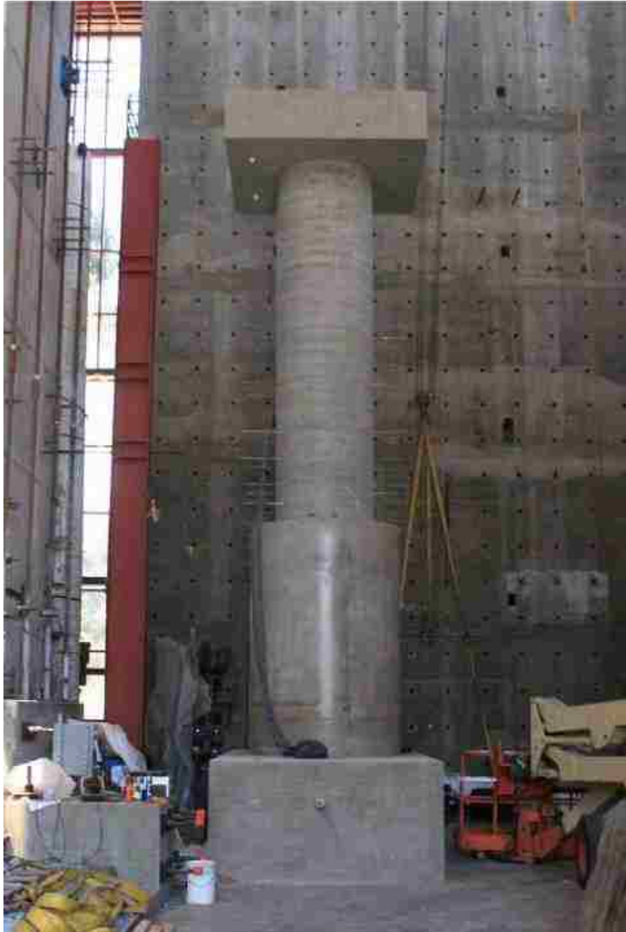
Figure 7-4. Cast-in-place column-shaft connection specimen (Murcia-Delso et al. 2013)
