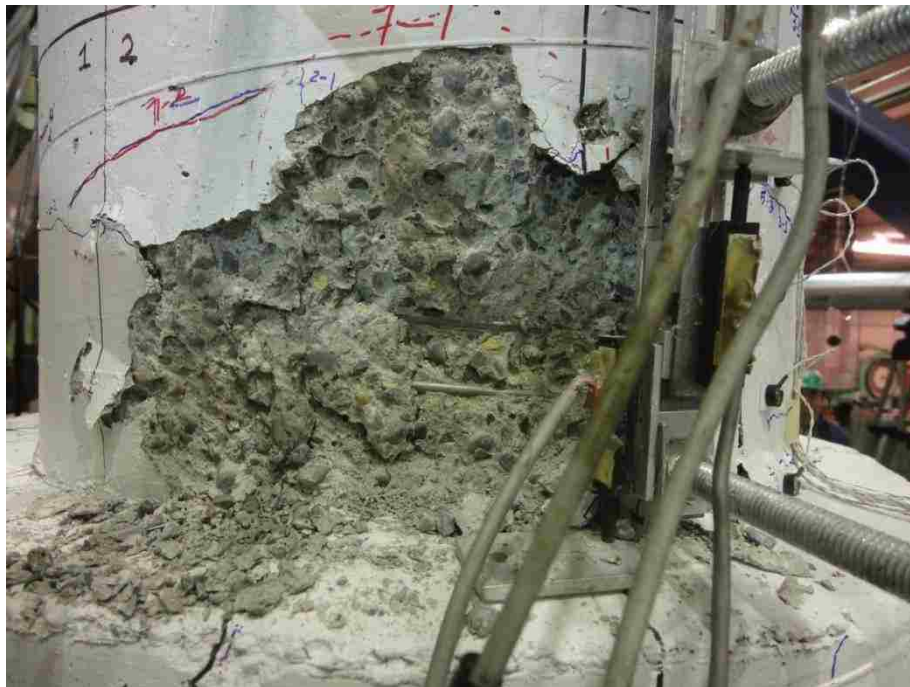
Figure C-0-16. DS-3 – Plastic hinge formed in the column at 4.57/-4.84 percent drift
